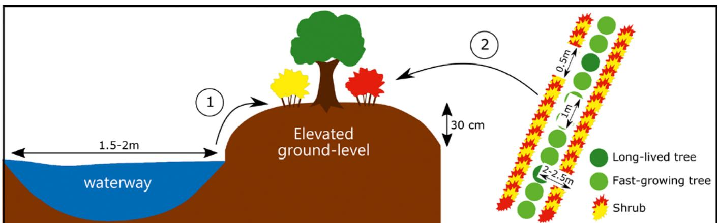
A waterway is created by digging out the soil and using it to raise the ground-level (1), where a new hedgerow is planted (2).
